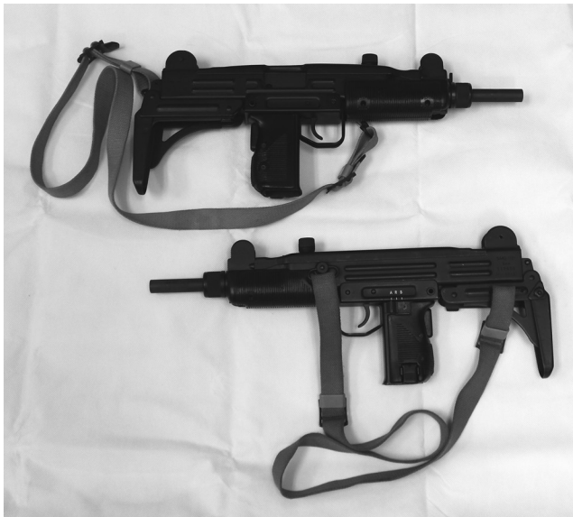
Figure 4.28 (See color insert.) The UZI submachine gun. The depicted examples were manufactured as submachine guns by Israeli Military Industries in Israel and are so marked on the left side of the receiver as UZI SMG. The English-marked selector switch is above the trigger, depicted in the lower example. Hebrew-marked selectors are also encountered. (Image from author's collection.)
